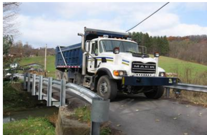
Live Load Test of Hackers Creek Bridge
