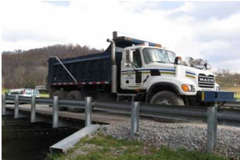
Live Load Test of Peel Tree Bridge
